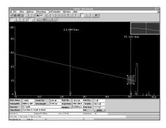
FMTAP version 3.1 OTDR trace analysis software allows you to access, analyze and document OTDR test data from a PC Windows platform. You can easily analyze single and multiple fibers and document the quality of fiber links in your network using FMTAP software and your saved OTDR data files.
